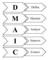
Fig. 9.12: DMAIC- Six Sigma Framework
