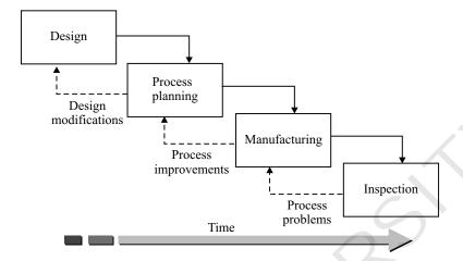
Fig. 3.1: Process Planning: Design And Manufacturing Interface (Source: Process Planning: The design/manufacture interface By Peter Scallan)
