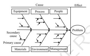
Fig 9.6: Fishbone Diagram
