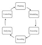
Fig. 11.2: Planned Maintenance Work Cycle
