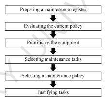
Fig. 11.3: Steps Involved in Developing a Maintenance Policy for Facilities and Equipment
