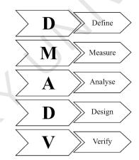
Fig. 9.13: DMADV- Six Sigma Framework
